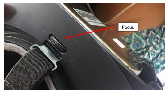
Figure 47- Location of the wheel to adjust focus
