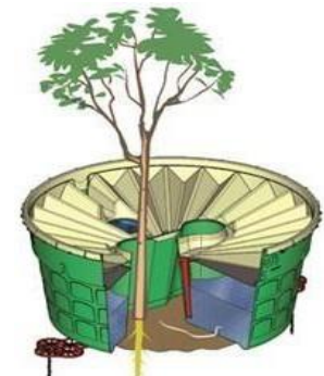
Figure 6-Diagram of Waterboxx showing wick positioning near plant roots
