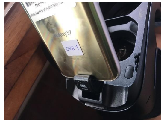
Figure 45-Placement of the phone into the flipped-up port
