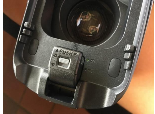
Figure 44- The point that should be slid and lifted
